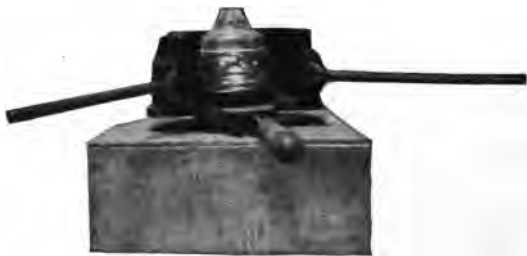
FIG. 89.—Lamp bowl blown in mold.
